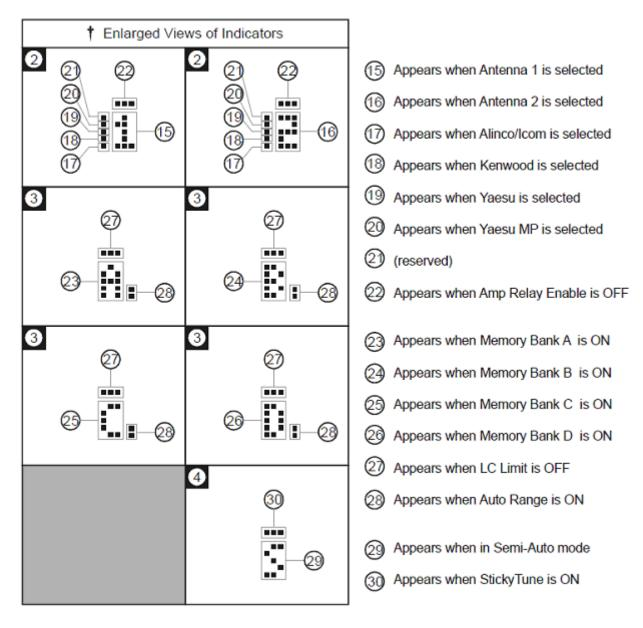
Figure 7 Display Tuner Indicators Enlarged
